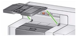
13. Open the printer access cover and remove the printer cover.
