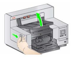
Loosen the thumbscrews on each end of the upper imaging guide and remove it from its position
