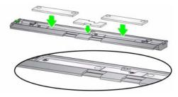
10. Install the drainage strip in place of the black strip that was removed in Step 8.
