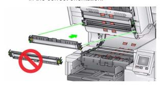
Loosen the upper flippable background accessory. Use the screwdriver provided to loosen all four thumbscrews.
