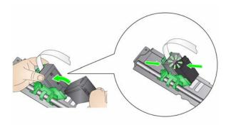
22. Rotate the printer carrier up and snap the ink cartridge in place.
