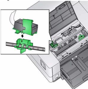
17. Connect the printer cable from the printer carrier to the left side of the printer circuit board. Be sure the copper side of the printer cable is facing down.
